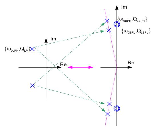
Can show that the upper hp pole maps to one upper hp pole and one lower hp pole as shown. Corresponding mapping of the lower hp pole is also shown
