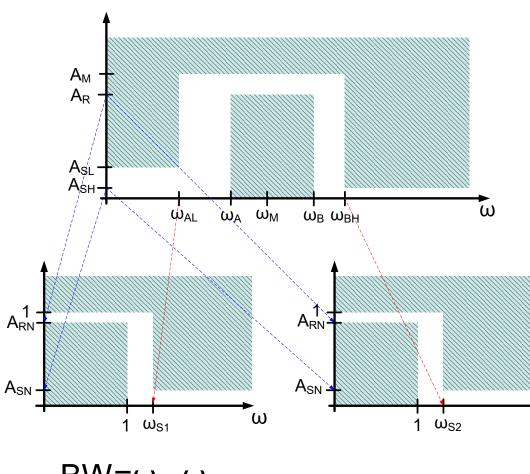
$BW = \omega_{\rm B} - \omega_{\rm A}$  $\omega_{\rm M} = \sqrt{\omega_{\rm B} \bullet \omega_{\rm A}}$
