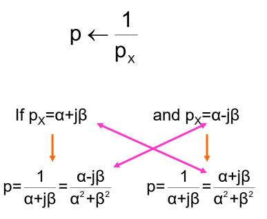
Highpass poles are scaled in magnitude but make identical angles with imaginary axis
