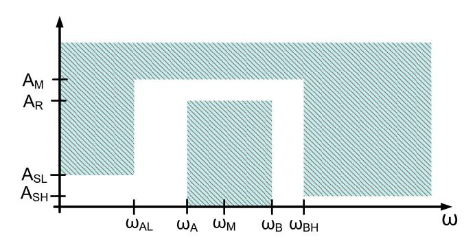
BW= $\omega_{\rm B}$ - $\omega_{\rm A}$  $\omega_{\rm M} = \sqrt{\omega_{\rm B} \cdot \omega_{\rm A}}$  In this example,
