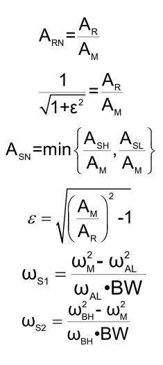
$\omega_{_{SN}} = \min\{\omega_{_{S1}}, \omega_{_{S2}}\}$
